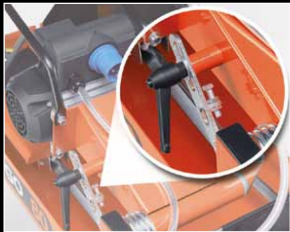
Adjusting screw to use diamond disk Ø 300 or Ø 350 mm.
